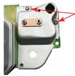
Install the gauge and housing assembly back into the cluster with the 2 previously removed screws
