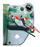
Install pink (C), and black (D) wires onto the gauge studs as shown
